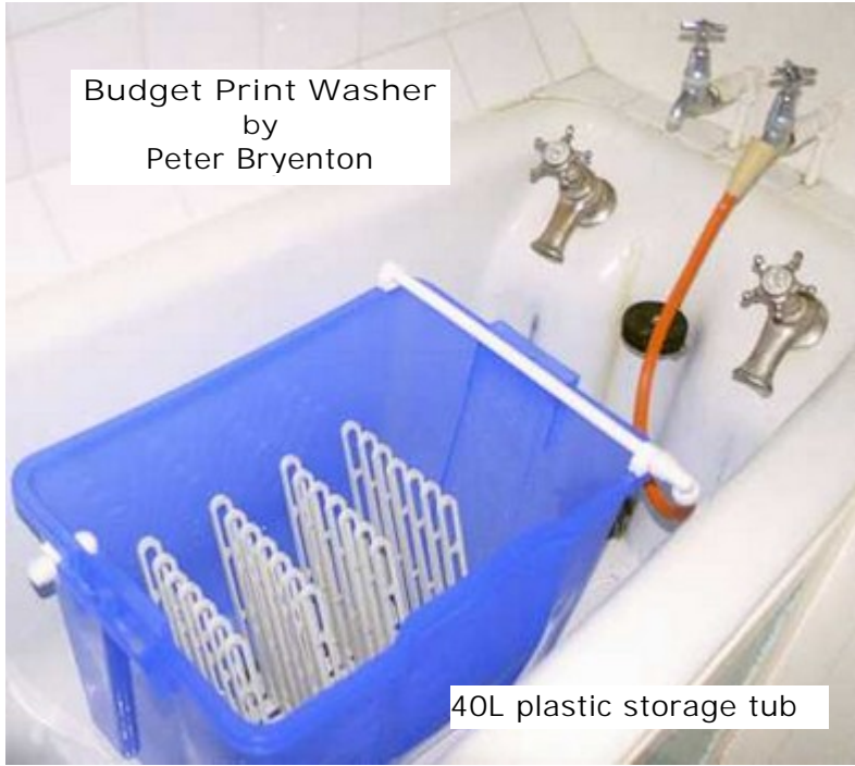
Syphon hose empties tank rapidly after use
