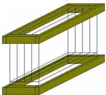
This diagram shows the box without the wood attached. The box is 10 1/4" high, 6 1/2" wide, and 11 1/2" long. There are 6 dividers making 7 compartments of 9"x11"x3/4" each. You can build your washer to whatever dimensions you want though.
