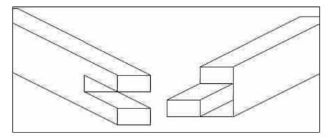
**tenon** - A way to join pieces of wood which increases the amount of wood surface for gluing. There are many kinds of tenons, this is an end to end tenon.
